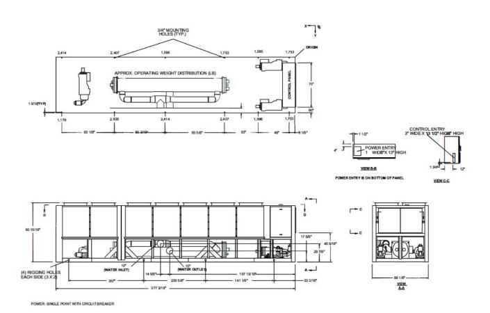
Minimum Clearances: Units Side by Side: 12 ft, Control Panel to Wall: 5 ft, Side to Wall: 8 ft, Front to Wall: 8 ft. Install unit on flat level surface.
