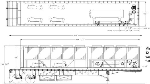
Minimum clearances: units side by side: 12 ft, control panel to wall: 5 ft, side to wall: 8 ft, front to wall: 8 ft. Install unit on flat level surface.
